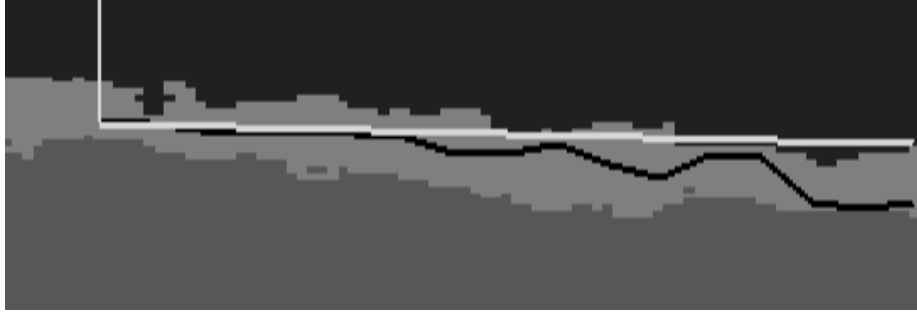
Figure 5 Vertical cross section with three layers in a shore-face reservoir and two possible well paths that are 4000m vertically. The light well path is determined only on the first observation of the middle layer, while the dark well path is determined also on an updated model for the layer for every 250m of the well path.
