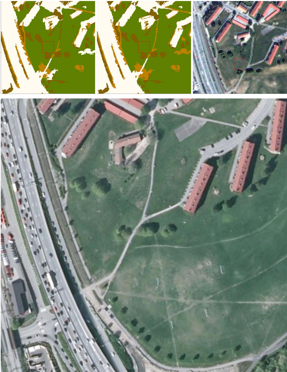
Figure 6. Assessment of classification result. Upper left: classification result. Upper center: edited classification result. Upper right: Pansharpened Quickbird image. Bottom: Aerial orthophotography.
