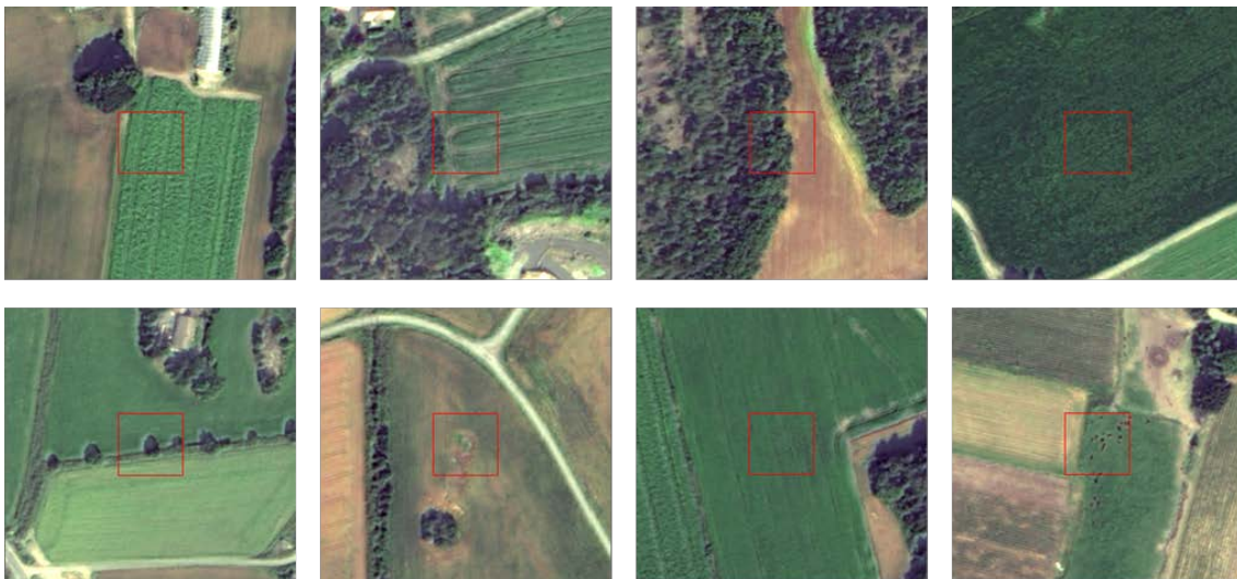
Figure 19. Examples of obvious misclassifications. Top row, from left: parallel wheel tracks plus some strong spots, turning wheel tracks, forest within agricultural mask, texture in field with other crop (e.g., potato). Bottom row, from left: single tree with shadow, field island, green cereal field, many single strong spots
