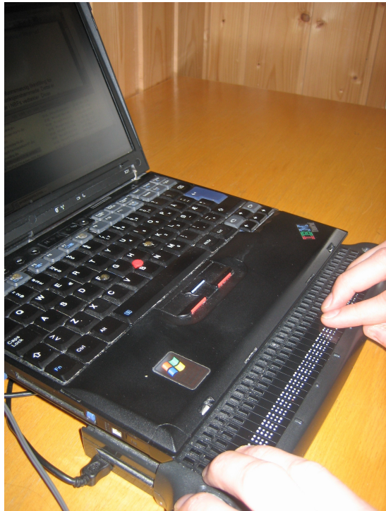
Figure 1: A laptop PC equipped with assistive technology; i.e., a hardware braille display and screen-reader software.
