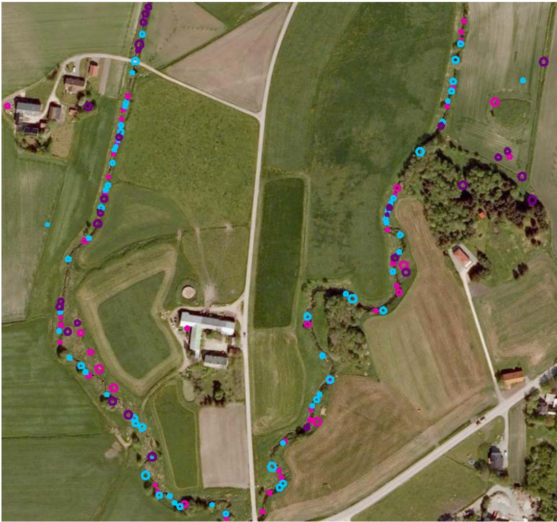
Figure 58. False pit detections, especially along ditches. Different colours denote different confidence levels.
